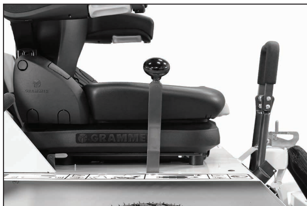
Correct FSC Lever Neutral-Park Position
