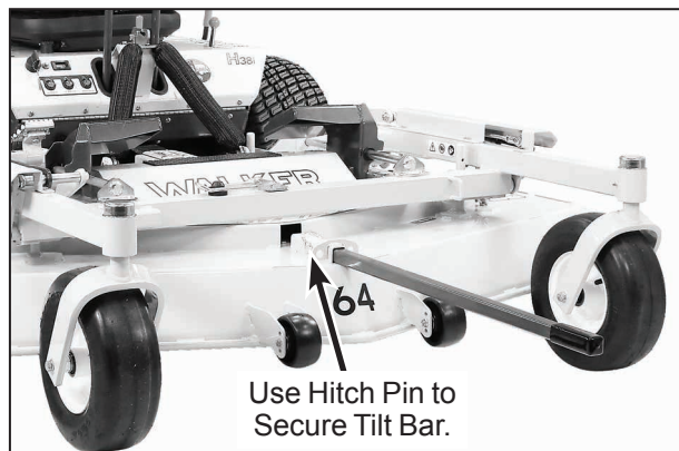
Tilt Bar Installed
